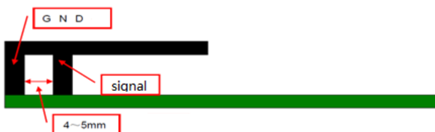
Figure 3-2 Location of signal point and earth point for PIFA antenna
